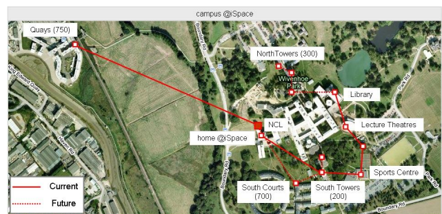
Figure 4: Fiber-to-the-Home (FTTH) connectivity
